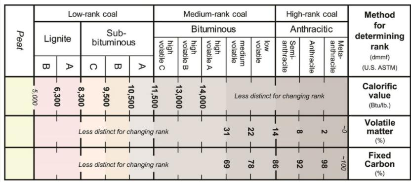
U.S. coal rank system showing the parameters used to define ranks.
